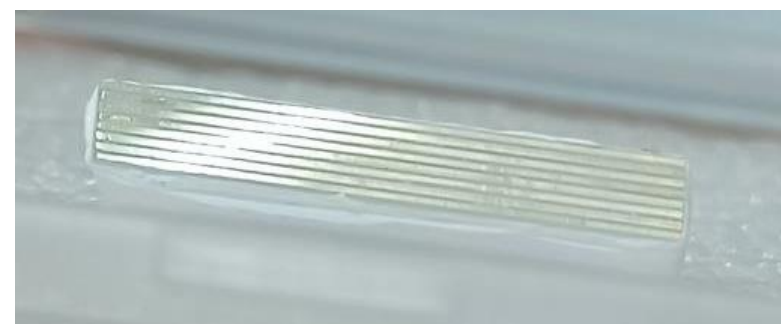
BGO-EJ232 Semi-monolithic Metascintillator
