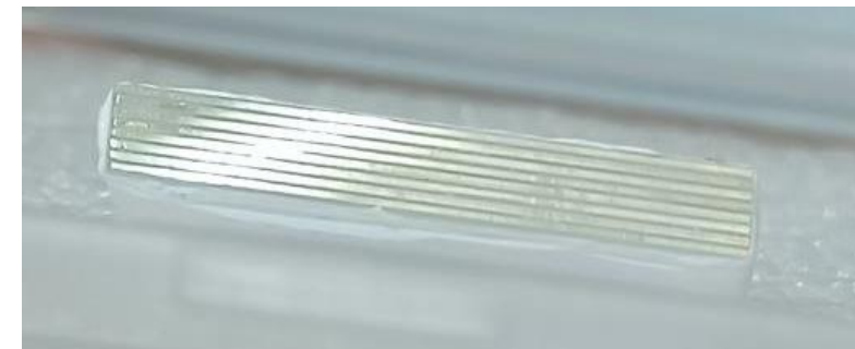
BGO-EJ232 Semi-monolithic Metascintillator
