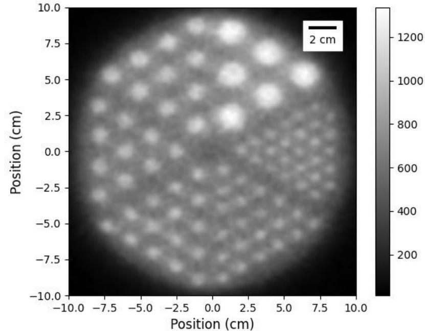
Derenzo brain phantom at 1/100th dose, using a TOPAS-simulated Pb-glass HGMT scanner
