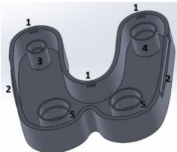
3D printed thyroid-shaped phantom filled with  $^{131}\text{I}$ -mIBG
