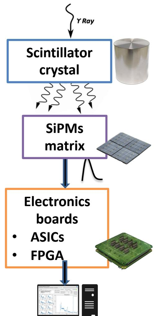
Gamma-ray detection module, based on a 2"  $\text{LaBr}_3(\text{Ce}+\text{Sr})$  scintillator crystal optically coupled with a matrix of 8x8 SiPMs. The SiPMs are read out by 4 custom 16-channels GAMMA ASICs and the data acquisition is managed by an FPGA.
