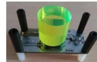
SiPM preamplifier board with EJ-276G scintillator
