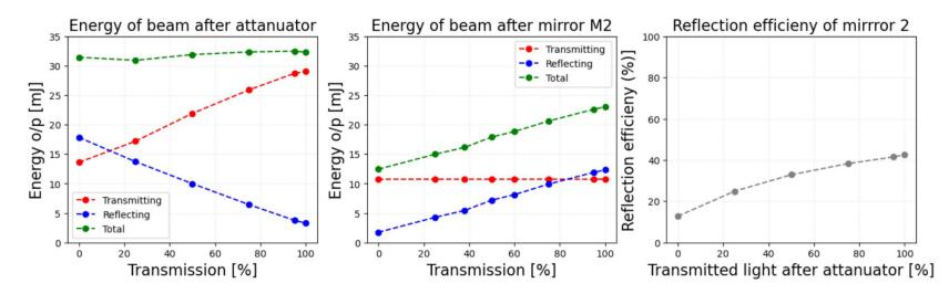
The total energy of the laser beam remains the same but the energy of p-polarised and s-polarised light varies with respect to the transmission through the attenuator. Unwanted light components in the infrared and green (base wavelength and 2nd harmonic) are transmitted through the mirror and ultimately absorbed on a beam dump.
