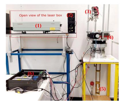
(1) Laser head, (2) Attenuator and mirror mount,
