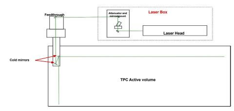
Schematic representation of SBND - UV laser calibration set up
