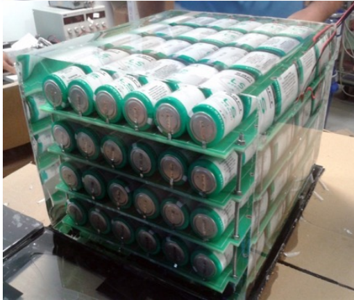
The cluster of 96 batteries covered by gel
