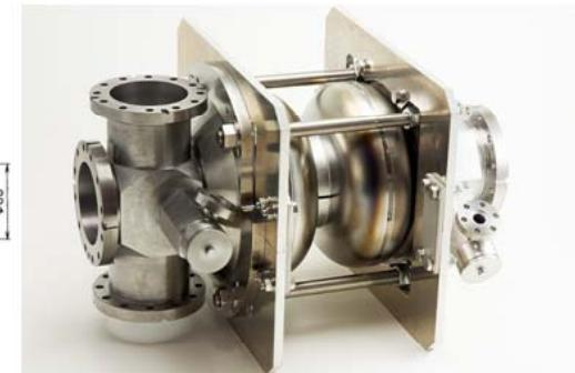
L-band 2-cell cavity for the injector
