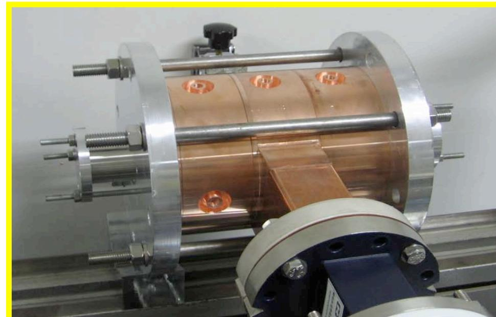
Deflecting-cavity under cold test
