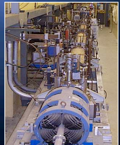
Linear accelerators At LLNL PLEIADES (to <150 MeV)
