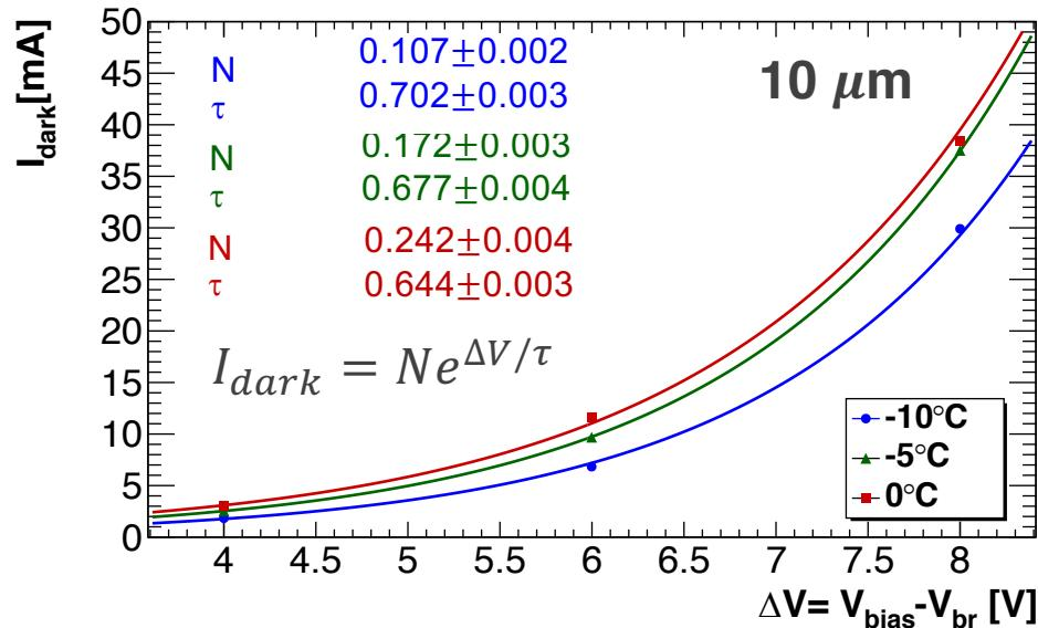
For the expected radiation level, **the best SiPMs choice is the 10 μm one** for its minor dark current contribution.
