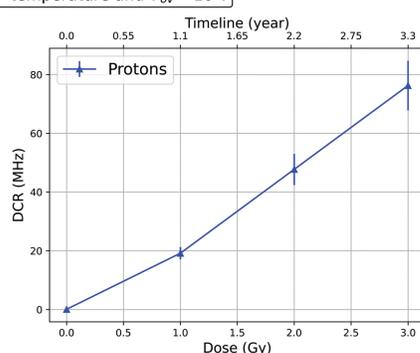
Inferred DCR per pixel for Terzina SiPMs sensitive area from IV measurement during the irradiation
