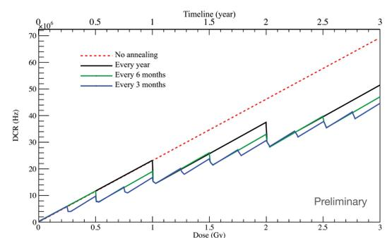
Different annealing cycles for the total DCR change during satellite lifetime
