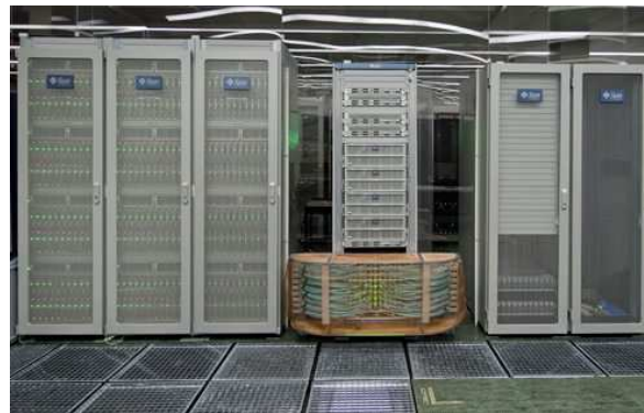
(f) The Schrödinger supercomputer at UZH, 4608 cores, 576 nodes 2× Xeon X5560 4C @ 2.8GHz RAM 24GB, 218KW, (2009)
