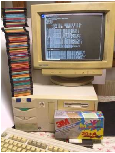
(a) Home: Pentium I 32-bit 133MHz RAM 16MB HD III 32-bit 1.6GB, (1996)
