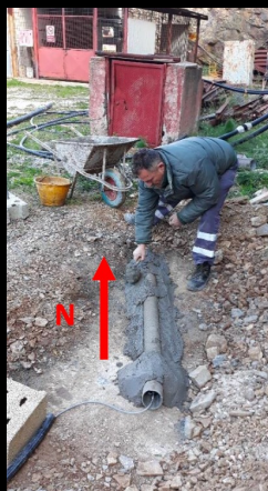
A magnetometer (N-S orientation) is located on surface
