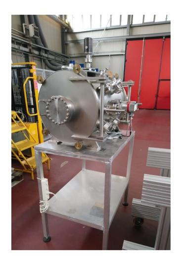
The 'pocket' cryostat is being instrumented in a dedicated space:
