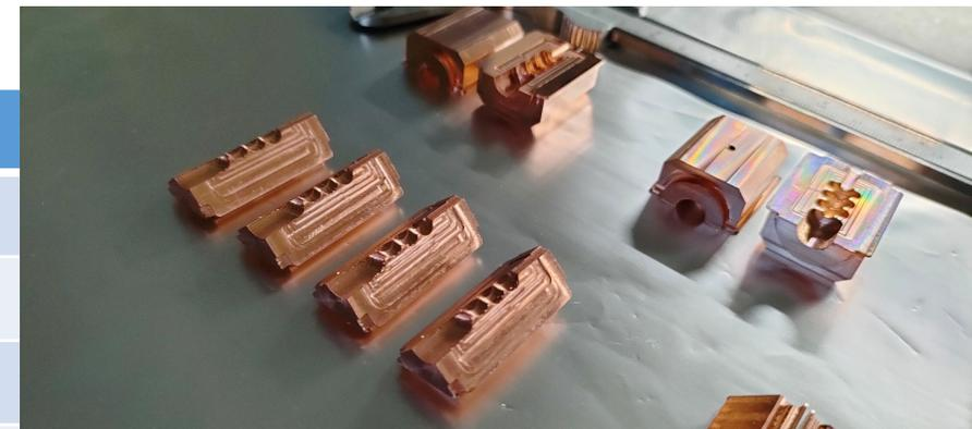
Machined sectors for 2-halves and 4-quadrants Cavities
