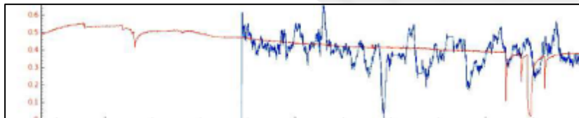
Target polarization during RGC experiment: P(\text{NH}_3) \sim 70\% , P(\text{ND}_3) \sim 50\%
