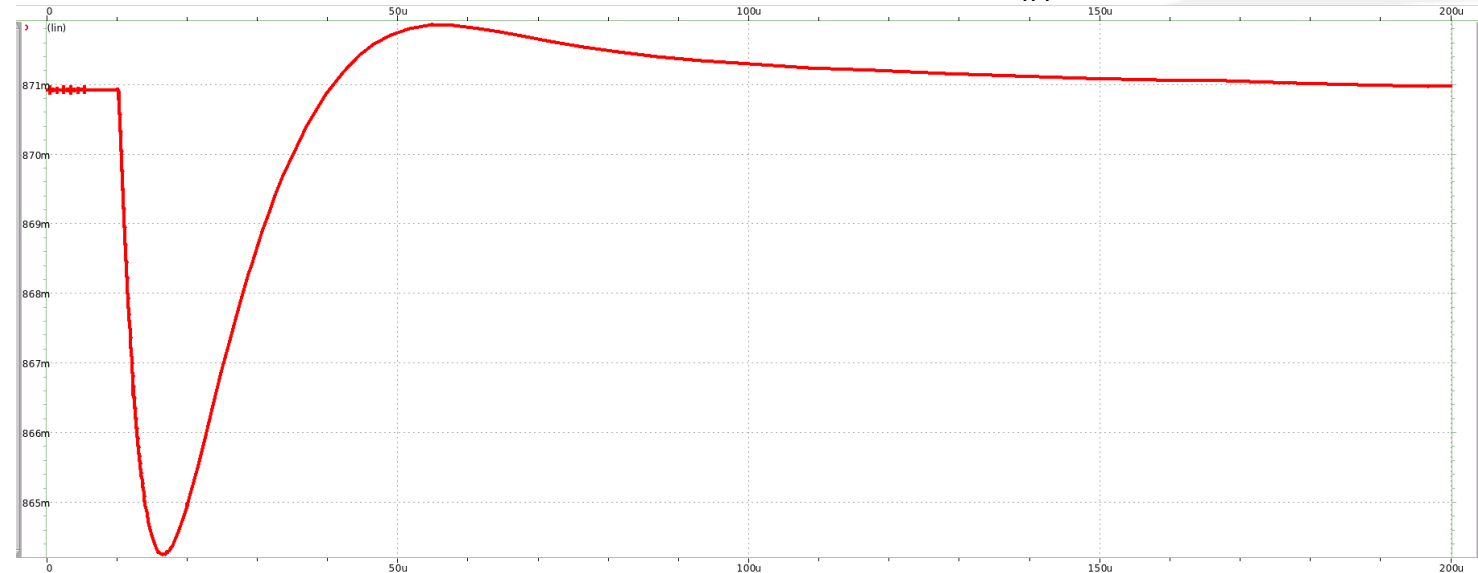
Simulated Shaper output ( Q_{in}=1.6 \text{ fC} )
