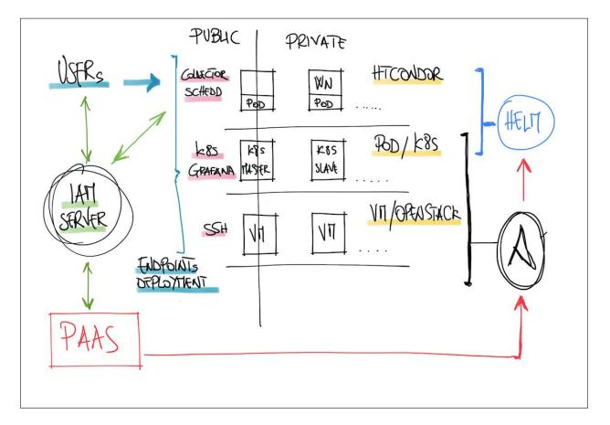
This deployment instantiate a k8s cluster which is then exploited to automatically deploy a working HTCondor cluster.
