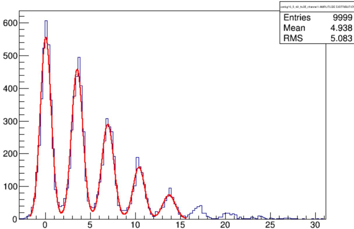
Amplitude distribution: Gain=  $(3.44 \pm 0.01)$  mV/pe
