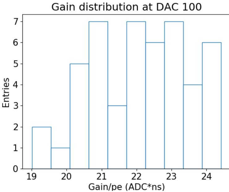
Gain measured at a fixed fine bias voltage DAC value (100) equal for all the channels.
