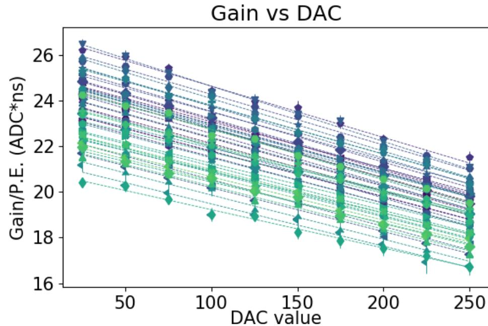
Gain vs SiPM fine bias DAC characteristics measured for all the SiPMs
