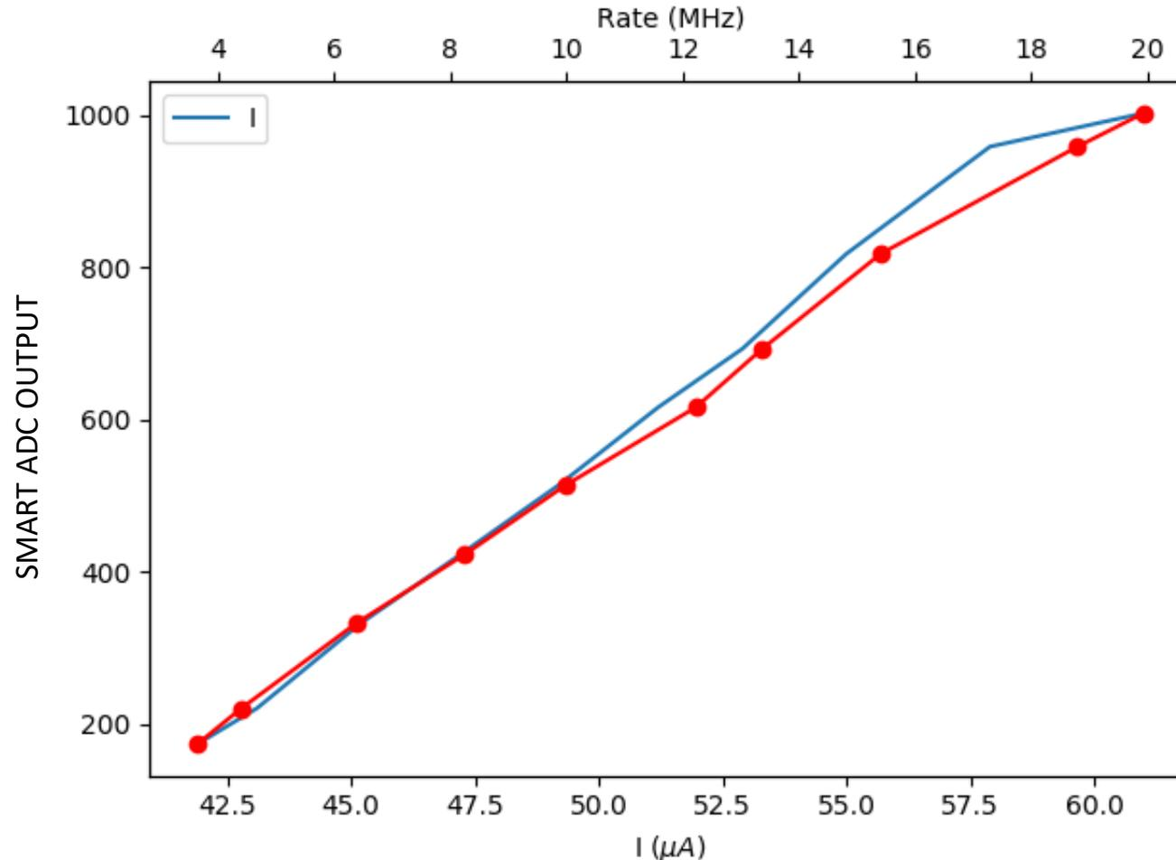
Slow-path measurements for a single channel, laser in continuous mode: max pulse rate: 20 MHz
