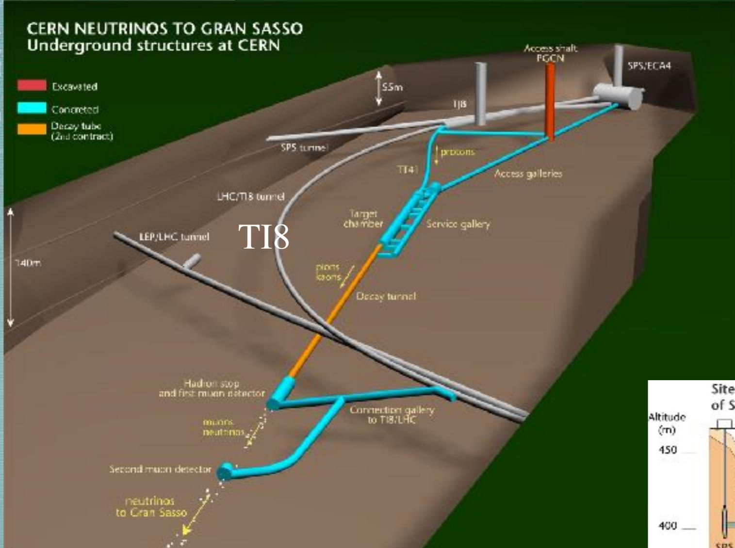
In orange, the decay tunnel where  $\pi$  and K from the CERN PS produce a neutrino beam towards Laboratori del Gran-Sasso (2006)
