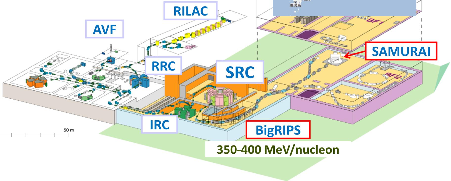
Intense (80 kW max.) H.I. beams (up to U) of 345AMeV at SRC
