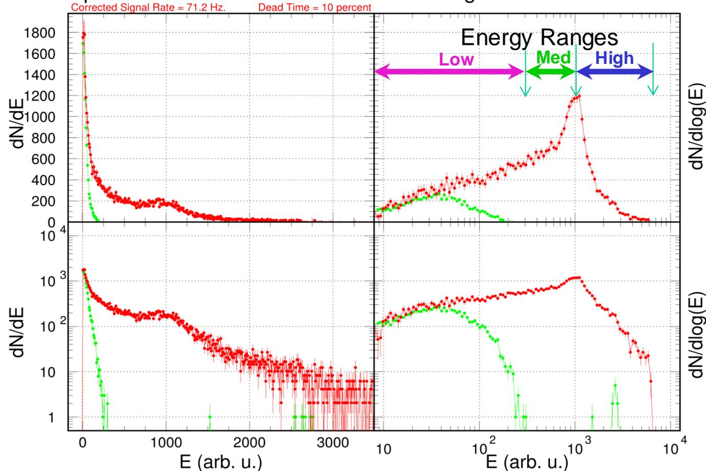
Typical example of a signal spectrum from the HPIC, accumulated in a 10 min time interval, and shown in all combinations of linear and log scales.
