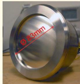
Xe-filled 70 181 by VacuTec ion chamber. View from the side of 50 μ stainless steel window.
