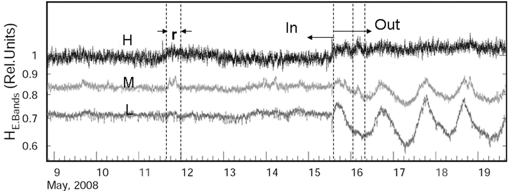
Initial operation of a SHPIC unit before introducing the SSTF-based noise subtraction. Left side (In) shows the detector behavior inside of an air-conditioned building and right side (Out) shows the records when detector was moved outside of the building
