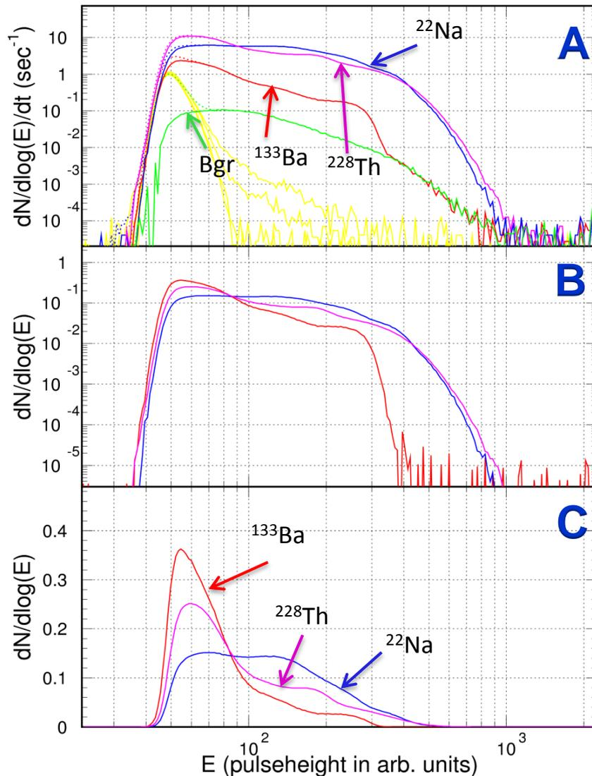
**A** - Irradiation of the Xe SHPIC in the lab using different low intensity radioactive isotopes with range of energies from 0.081 to 2.61 MeV. Green distribution shows natural background including cosmic radiation in the room. Yellow distributions illustrate the noise contributions measured using our SSTF method.
