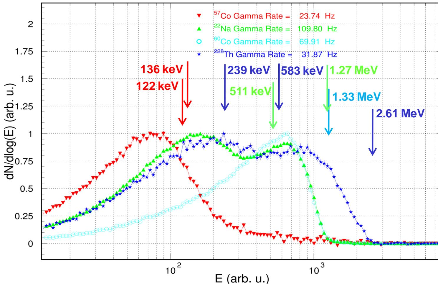
Irradiation of the Argon-filled SHPIC in the lab using different low intensity radioactive isotopes with range of energies 122 keV – 2.61 MeV
