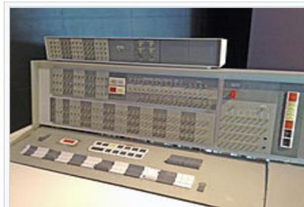
IBM 7094 operator's console showing additional index register displays in a distinctive extra box on top. Note "Multiple Tag Mode" light in the top center.
