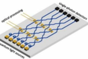
use particles of light to carry and process information. Qubits realised by processing states of different modes of light through both linear (mirrors, beam splitters, phase splitters, ...) and nonlinear element (quantum microprocessor based on laser photonics at room temperature)
