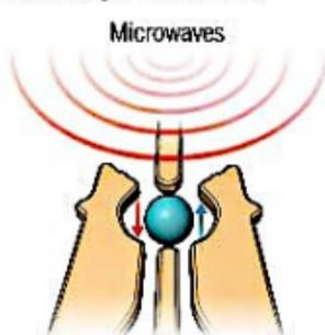
These “artificial atoms” are made by adding an electron to a small piece of pure silicon. Microwaves control the electron’s quantum state.
