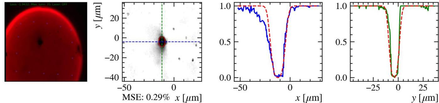
**Differential geometry techniques** used to correct for optical aberrations and measure the spot size and profiles.
