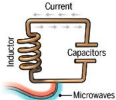
A resistance-free current oscillates back and forth around a circuit loop. An injected microwave signal excites the current into super-position states.
