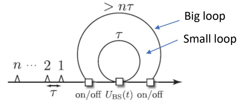
Example of a network with 3 inputs and a depth of 3 steps (3-1 Big loops): the input switch selects 3 pulses, since the time of the Small loop is exactly equal to the time between two pulses, the pulses enter the BS simultaneously. After a number of Small loops equal to the number of selected pulses, the pulses are sent to the Big loop, which returns them to the entrance of the Small loop.
