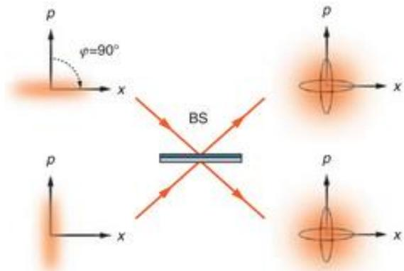
With the **loop** architecture, it's possible to increase the number of BS in the network simply by increasing the number of input pulses without changing the system's structure. Furthermore, in the loop structure, there's only one BS, so all the BSs in the network are identical.
