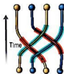
Quasiparticles can be seen in the behavior of electrons channeled through semiconductor structures. Their braided paths can encode quantum information.
