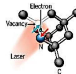
A nitrogen atom and a vacancy add an electron to a diamond lattice. Its quantum spin state, along with those of nearby carbon nuclei, can be controlled with light.
