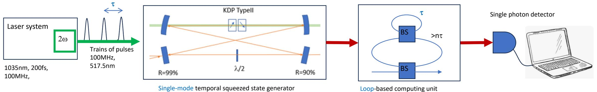
The **Gaussian Boson Sampling (GBS)** involves sending squeezed states into a network of beam splitters (BS) and measuring the photon distribution at the output. The beam splitter network 'entangles' the qubits (squeezed pulses), making the problem hard (ideally, the computational complexity grows exponentially with the number of qubits).
