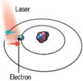
use the energy levels of electrons in neutral atoms or ions as qubits. In their natural state, these electrons occupy the lowest possible energy levels. Using lasers, we can “excite” them to a higher energy level. We can assign the qubit values based on their energy status
