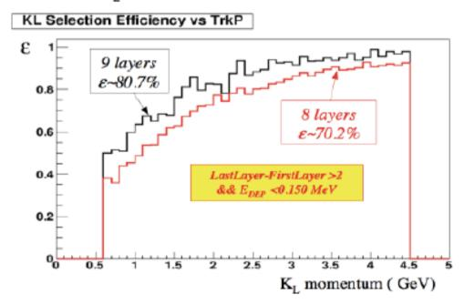
Performed a Very Loose  $K_L$  selector to compare configuration with 8 and 9 active layers  $\rightarrow$  Configuration with 9 layer gives better  $K_L$  efficiency
