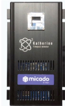
Housing of Timepix3 and Katherine readout. Housing dimensions are 13cm x 20,4cm x 3cm.
