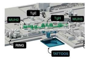
To increase the capture and the transmission of surface muons, the two HIMB beamlines will be based on solenoidal elements.
