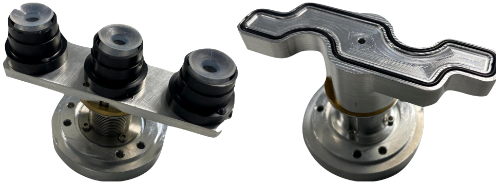
Figure 81: Original (left) and redesigned (right) spreader tool in use at Oxford.
