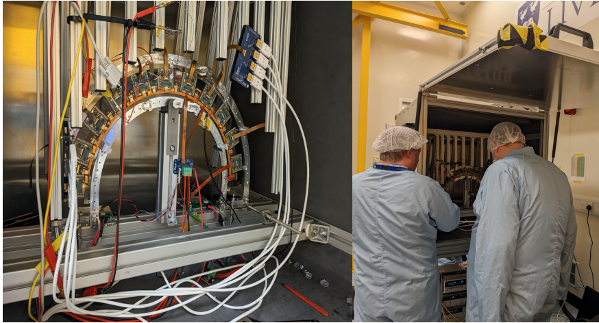
Figure 117: Ring 1 located in its test position inside the test box (left). The Liverpool test box, in its open position, with the lid open, allowing access (right).
