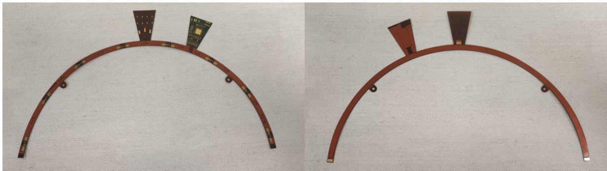
Figure 17: Left: front side of the v6 bus tape. Right: back side of the v6 bus tape where the three pads for the grounding connection are visible.
