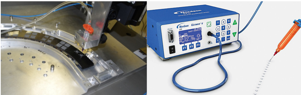
Figure 57: Left: gantry syringe mount. Right: Nordson fluid dispenser.
