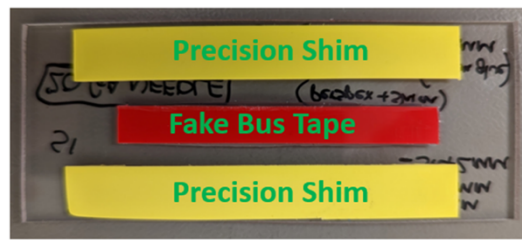
Figure 30: Fake bus tape and shims prepared for gluing onto Perspex
