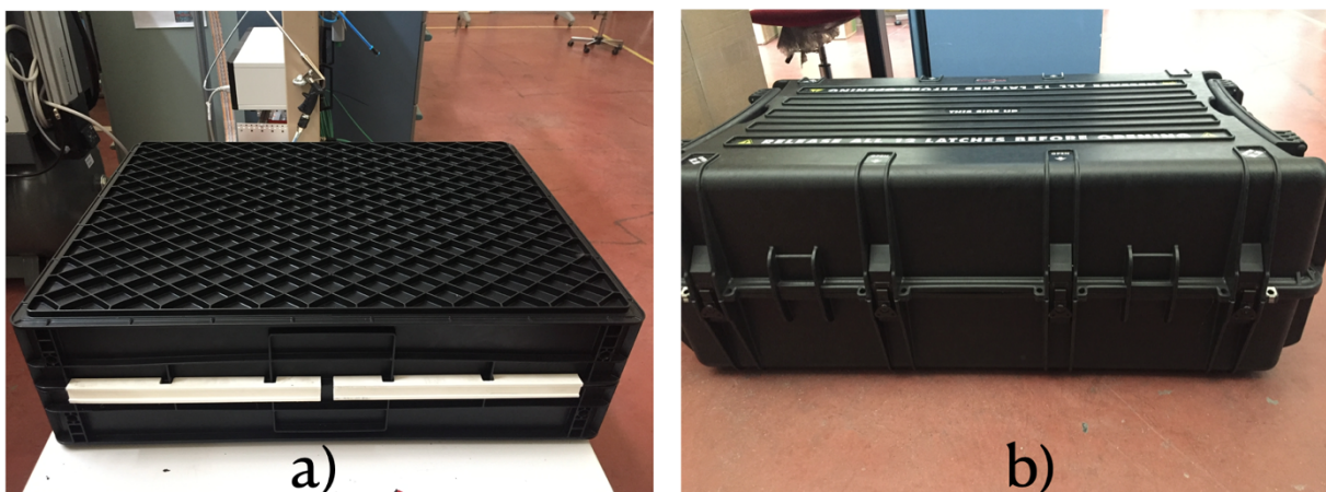
Figure 142: a) stacked commercial storage boxes for containing a half-ring in its protective Perspex plates. b) commercial hermetic box to contain one or two storage boxes for transport.
