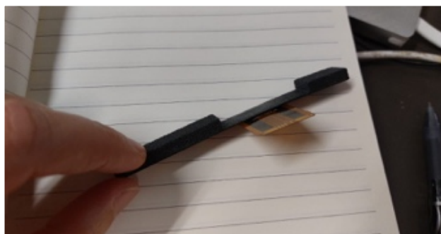
Figure 49: Sample with mini-tapes and pigtails glued on a bespoke mini-structure of prepreg and carbon foam. The carbon foam layer is minimized under the irradiation region to avoid possible irradiated powder to be missed and to minimize the material.
