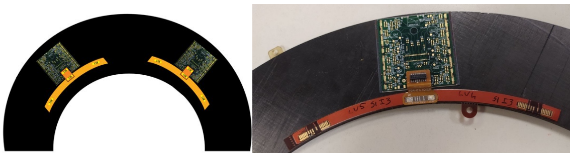
Figure 42: Left: Sketch of the Layer-2 half-ring with the two test samples done with a module connected to a piece of tape. Right: picture of one of the samples.
