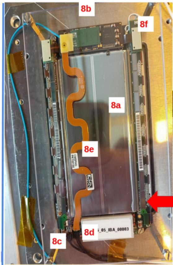
8) Encapsulation (8a) of the wire bondings with Sylgard, vtRX+ connector (8b), HV (8c), LV (8d), power tail (8e), soldering of the 2.5V wire (8f),
