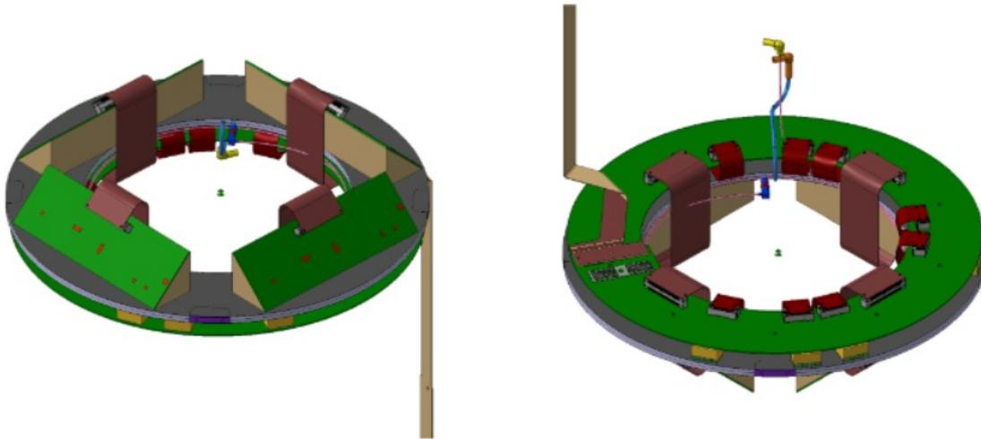
Bottom (left) and top (right) 3D models of the BCMp station including the aPCB ring
