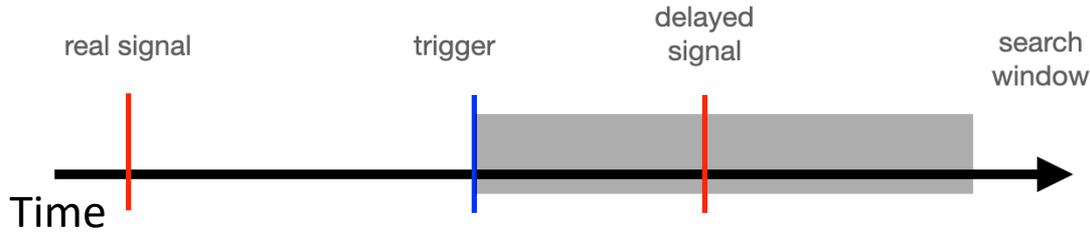
Predictable timing between arrival of data signal and trigger
