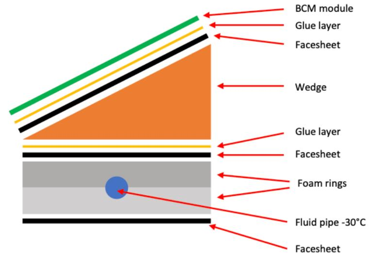
Cut view of the model (normal to module's length)
