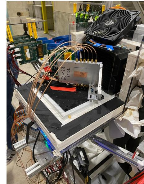
TB telescope and DUT
