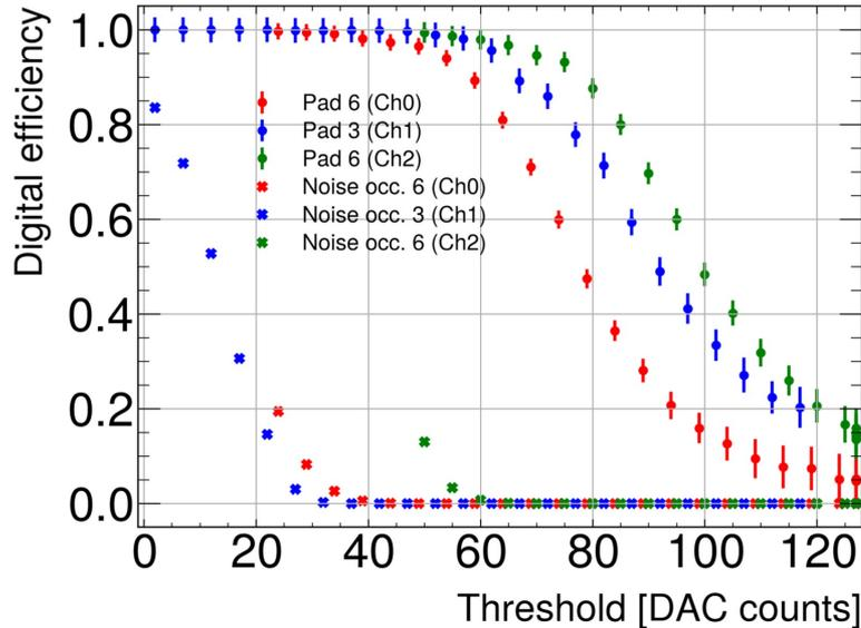
Calypso ver. C, S8 pCVD diamond, Pad 3, Cr/Au met., -1000 V, CFD threshold 52 DAC
