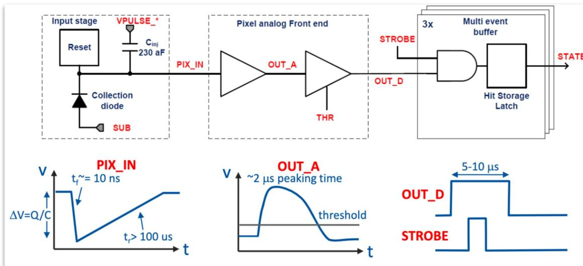
Pixel signal amplified and digitized at pixel level:
