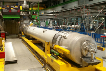
via HL-LHC technology 12 T Nb 3 Sn quadrupole
