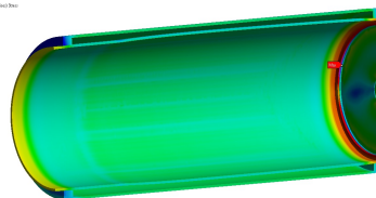
Simply supported vessel – stress field
