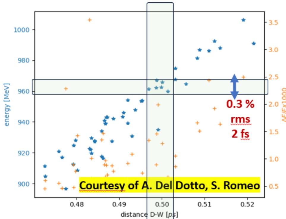
Results obtained by means of start to end simulations taking into account state of the art jitters in conventional RF photoinjector
