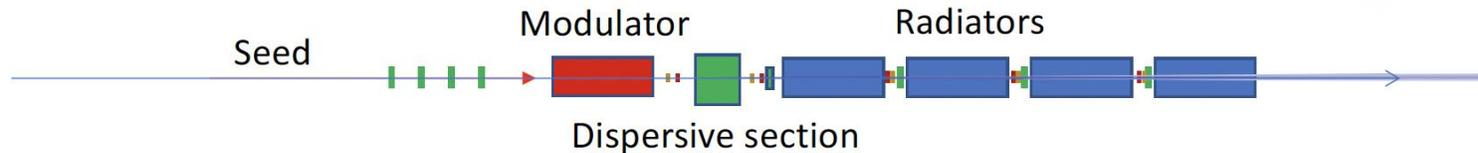
**SEEDED FEL** – Modulator 3 m + 4 Radiators APPLE II – variable pol. 2.2 m each – SEEDED in the range 290 – 430 nm (see former presentation to the committee and *Villa et al. ARIA—A VUV Beamline for EuPRAXIA@SPARC\_LAB. Condens. Matter 2022, 7, 11.*) – Undulator based on consolidated technology.
