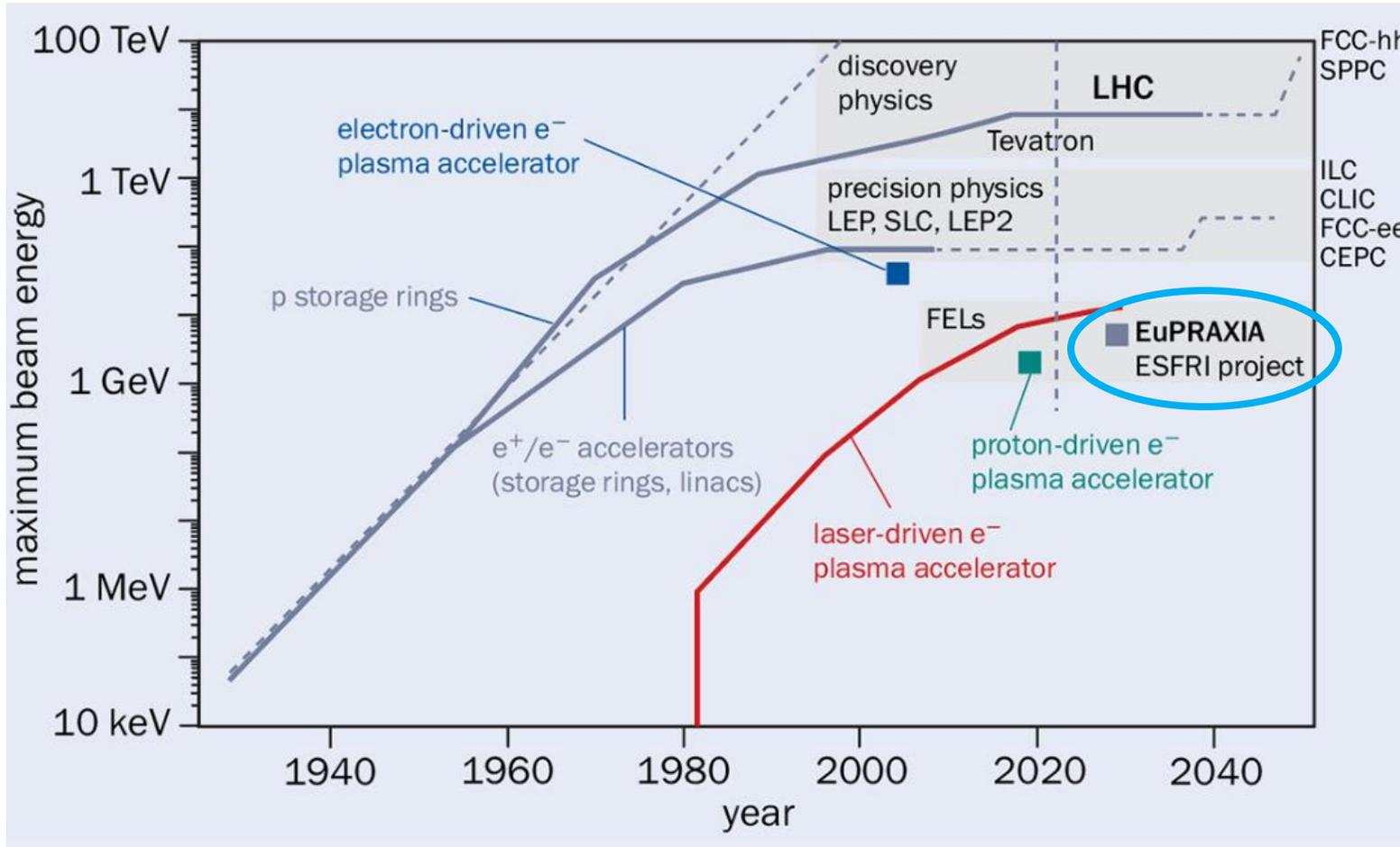
Updated Livingston plot for accelerators, showing the maximum reach in beam energy versus time. Grey bands visualize accelerator applications
