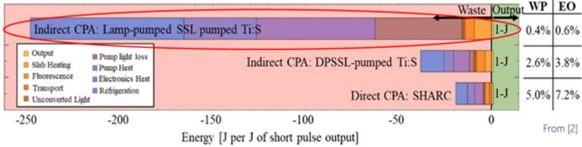
One of the main bottlenecks is the repetition rate of the laser driver (and poor efficiency)
