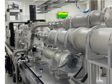
Beam transported to adjacent room where it is frequency doubled and then injected in the Ti:Sa Amplifier
