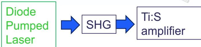
Improved efficiency and pulse rate if pumped with high energy, high pulse rate DPSSLs + advanced cooling schemes
