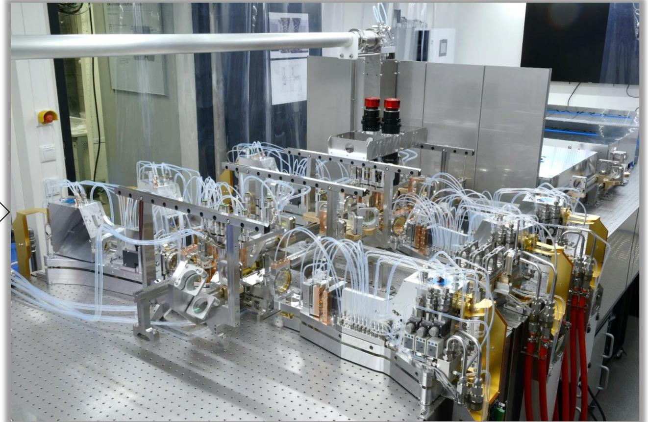
2017: 500 W extracted power per gain module
