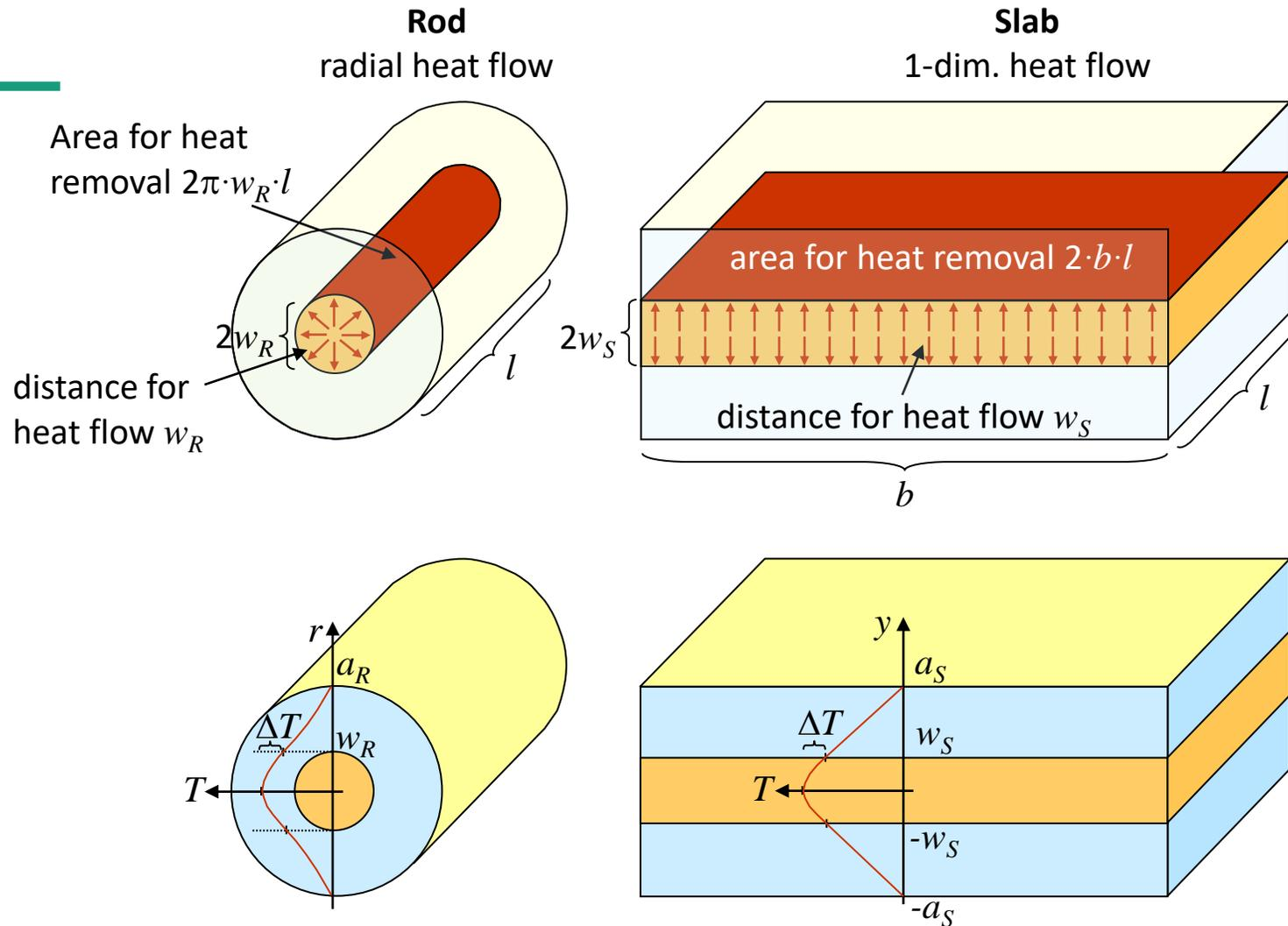
The phase difference  $\Delta\phi \sim \Delta T \cdot l$  determines the thermal aberrations and limits the power at diffraction-limited beam quality.
