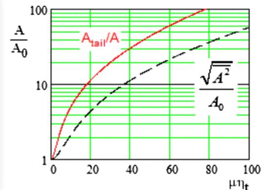
Tail and rms amplitude growth versus betatron phase advance times normalized transverse wakefield strength. Image credit: Ref. [3]
