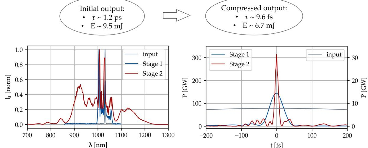
Fig 3: Measured spectra for each compression stage (left) and corresponding FROG-retrieved temporal profile (right). The output of the first compression stage is shown in blue, the one of the second in red. The initial laser output is depicted in grey. After the second compression stage a peak power > 300 GW is reached.
