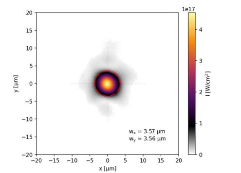
Fig 7: Measured laser focal spot and relative intensity profile at the interaction point. The gaussian fitting (in red) shows a circular spot with 3.5  $\mu\text{m}$  radius.
