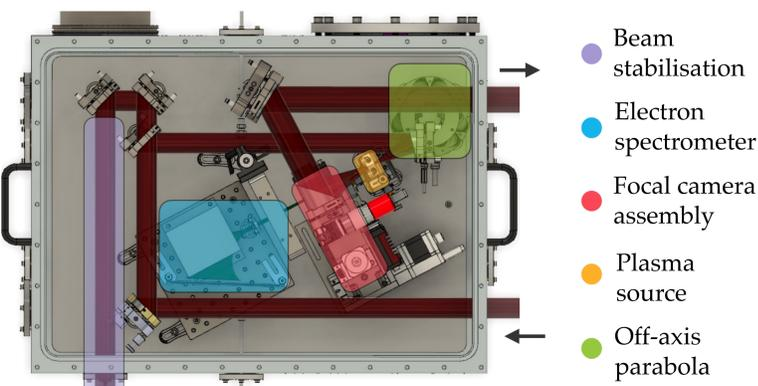
Fig 4: Scheme of the acceleration chamber. The main parts of the setup are enlighten in different colours.
