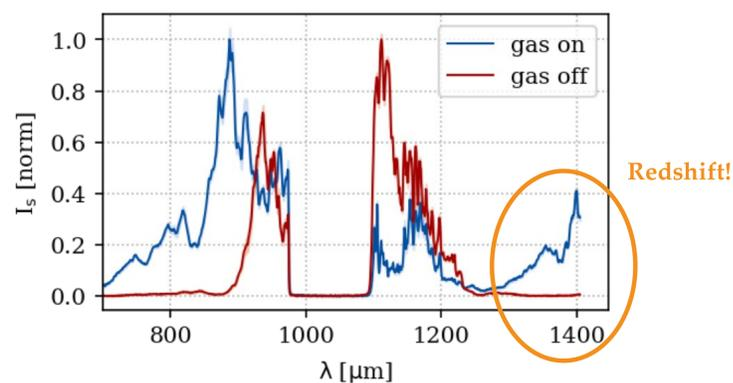
Fig 6: Laser spectra after the interaction point. The central wavelength (1030nm) has been filtered out for better visibility. The spectrum after the laser-plasma interaction (blue) is compared to the initial laser spectrum (red). Spectral shifts on both sides of the spectrum are evident.
