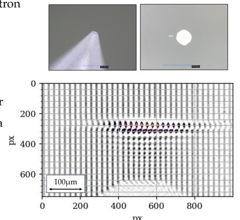
Fig 5: A typical interferogram used for the plasma density characterisation. The glass de Laval nozzle, visible on the bottom, has an output diameter of only 120  $\mu\text{m}$  and a throat of 40  $\mu\text{m}$ , as shown in the microscope images on top.
