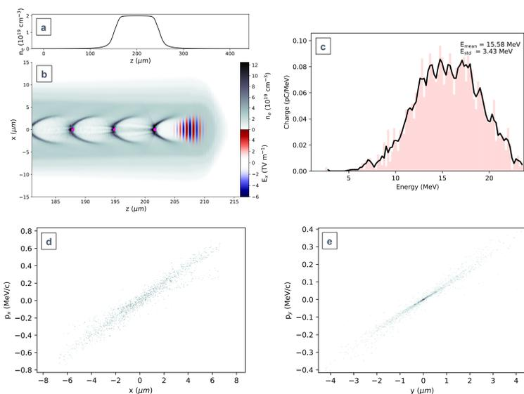
Fig 2: PIC simulation (FBPIC) showing the obtainable electrons parameters with a 6 mJ, 10 fs pulse. Panel (a) represent the plasma density profile along the propagation direction, panel (b) shows the wake evolution and the injected electrons (pink), panels (c), (d) and (e) depict the obtained electron spectrum at the end of the propagation (~100  $\mu\text{m}$  after the source) and the x-y phase space.
