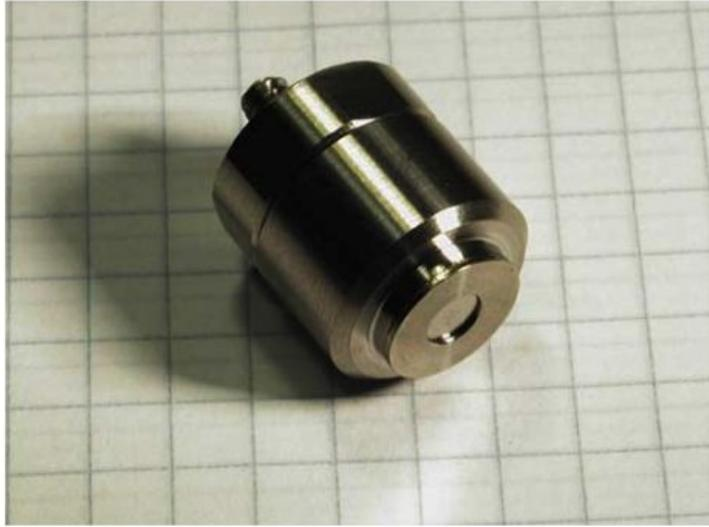
Fig. 3. The closed capsule (small design). The welding of the front ring is visible. The post has got a 6-32 UNC thread with a length of 6.3 mm.
