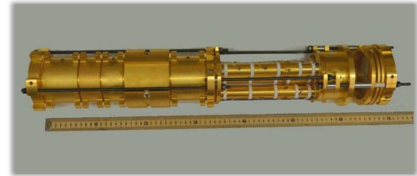
A multi-cell trap for increasing positron beam rate
