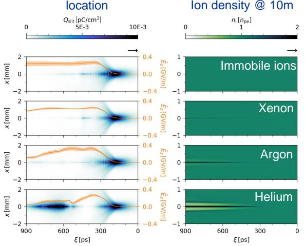
Ponderomotive force of the wakefields causes ion motion  $\rightarrow$  more significant later in the bunch (more time and higher wakefield amplitudes)
