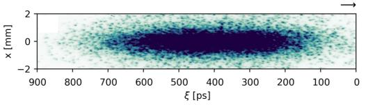
3.5 m of vacuum propagation downstream the plasma exit. Approximately Gaussian in longitudinal and transverse direction
