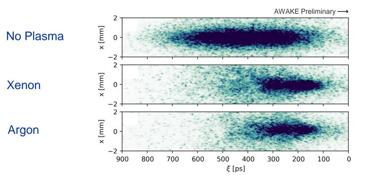
$n_p = 3 \times 10^{11}$  protons per bunch  $n_{pe} = 4.8 \times 10^{14}$  cm<sup>-3</sup>
