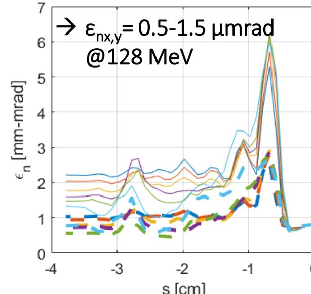
Evolution of the *energy, energy spread and emittance* in the plasma stage for the witness for different witness-driver delay. The maximum energy gain is of about 1.0 GeV/m as measured
