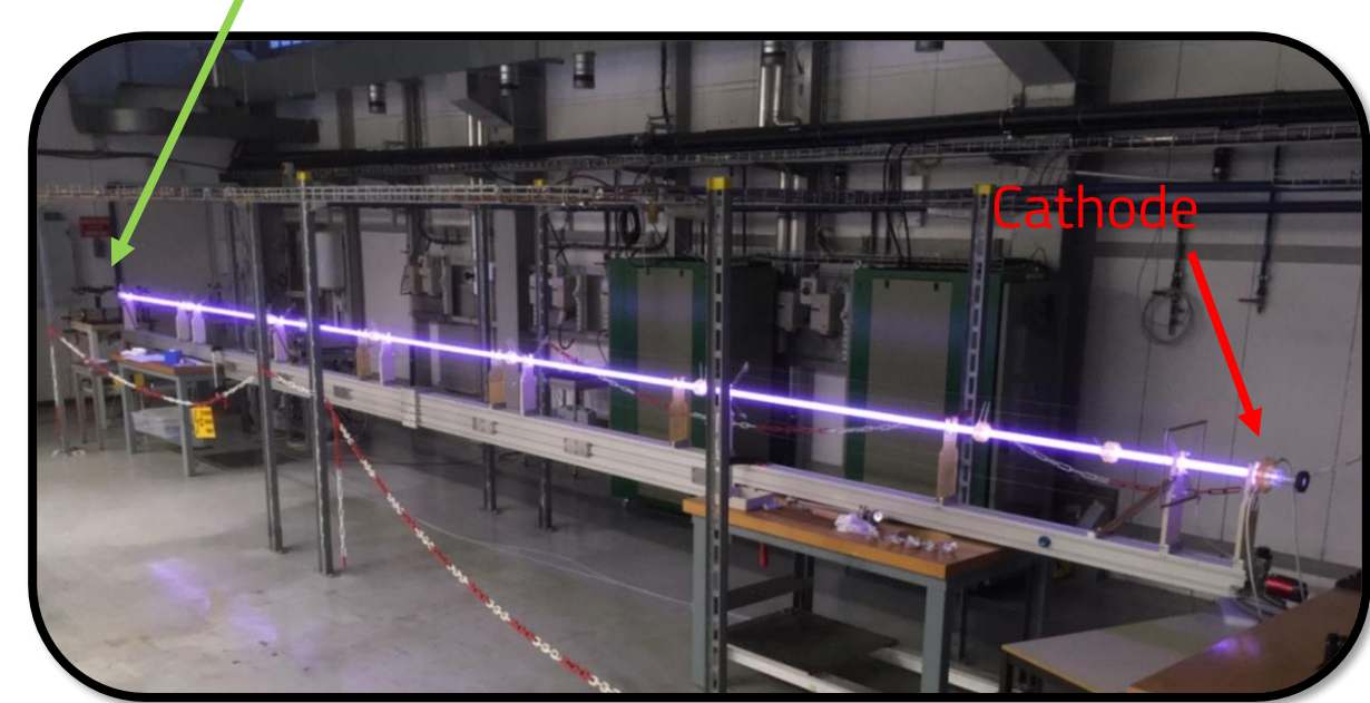
10 m single plasma, 24 Pa Ar, ignition+heating 500 A, ~30 us pulses
