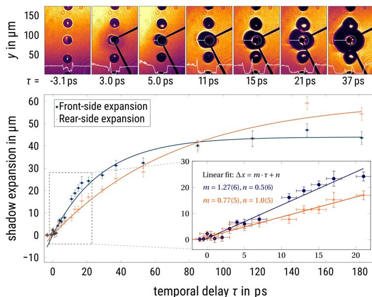
Fig. 2: Expansion of the front (blue) and rear (orange) of the plasma parallel to the laser propagation axis as a function of the delay  $\tau$  [1].
