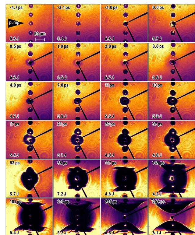
Fig. 1: Shadowgraphic images of water droplets with coronagraph for different pump-probe delays  $\tau$  (top left). The laser energy  $E$  on the target is also shown (bottom left) [1].
