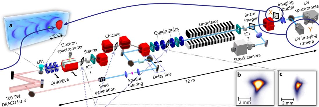
**Virtual diagnostics** provide data from all imagers in a digital form with access to the phase space of the beam in the beamline
