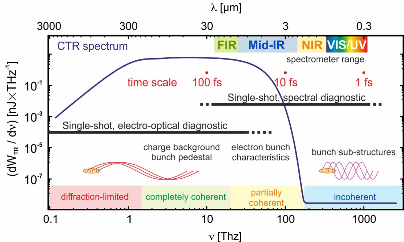
Sim: 200 MeV, 20pC, 10 fs bunch length, 20  $\mu\text{m}$  diameter
