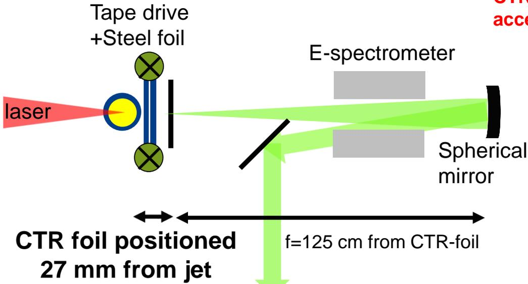
CTR-spectrometer acceptance angle  $\theta \sim 16$  mrad
