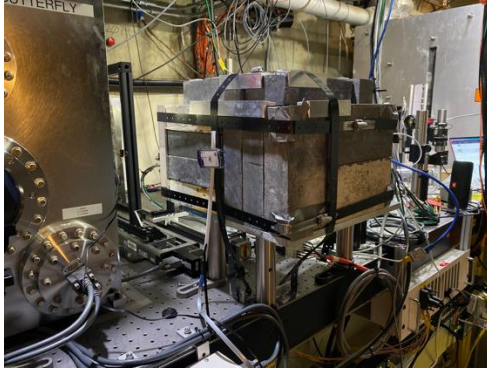
shielding to keep ePix safe during “high radiation times”
