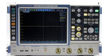
Oscilloscope Rohde&Schwarz RTO1044 (4 Ghz BW - 20 Gsa/s)
