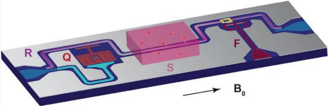
*Proof of concept of a spin-based quantum memory for superconducting qubits.*
