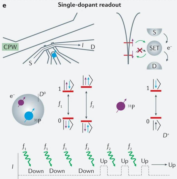
Readout of shallow dopants using the DC current  $I$  running through a single-electron transistor (SET) charge sensor. Dopant energy levels ( $D^+$ ) and ( $D^0$ ) form the two-level system for the ionized nuclear spin and the electron spin qubit, respectively. Transitions are addressable using distinct frequencies ( $f_1$  and  $f_2$ ) delivered via a coplanar waveguide (CPW).
