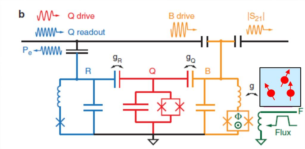
The resonator has an embedded superconducting quantum interference device (SQUID) and flux line (F) to allow for frequency tunability. This particular device implements a quantum memory, where quantum states from Q are transferred to S via R. [Y. Kubo et al. Phys. Rev. Lett.107, 220501 (2011)]
