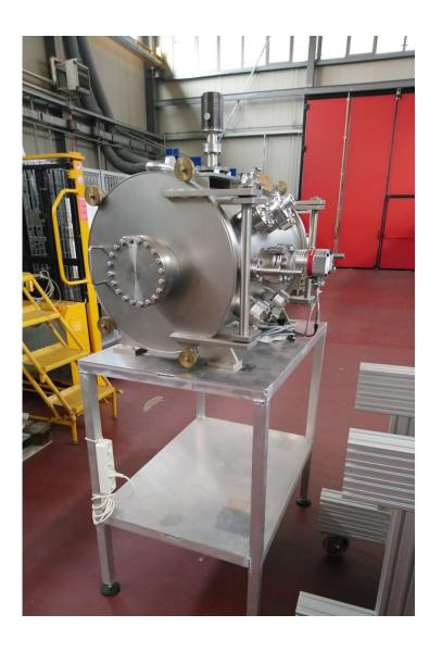
The 'pocket' cryostat is being instrumented in a dedicated space:
