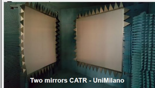
Creation of collimated beam and Quiet Zone for DUT
